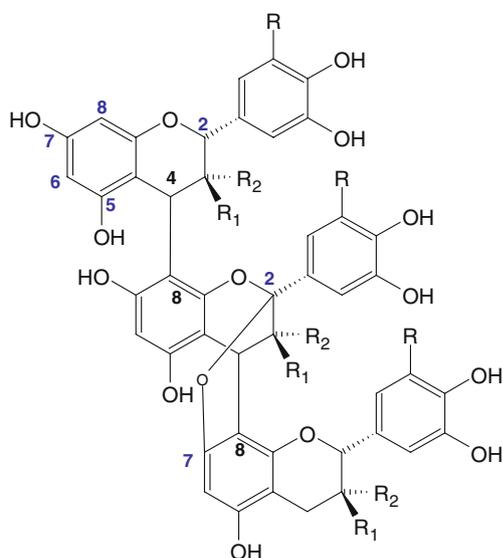
**Fig. 1** Structure of condensed tannins. Flavanol monomer units can be linked by C4–C8 bonds (*upper unit*), C4–C6 bonds (not shown) or both a C4–C8 and an ether C2–O–C7 bond, also called A-type bond (*lower units*). A-type bonds are present for instance in native cranberry tannins
