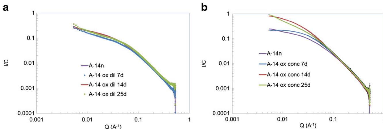
**Fig. 5** Kinetics of oxidation followed by SAXS: SAXS intensity (normalized by concentration) of oxidized tannins in dilute (a) and concentrated (b) solutions, in the log  $I$ -log  $Q$  representation
